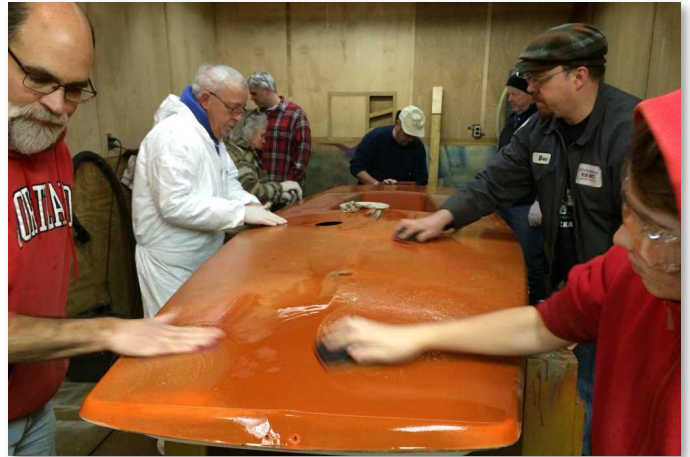
The deck is wet sanded in preparation for filling and priming.
