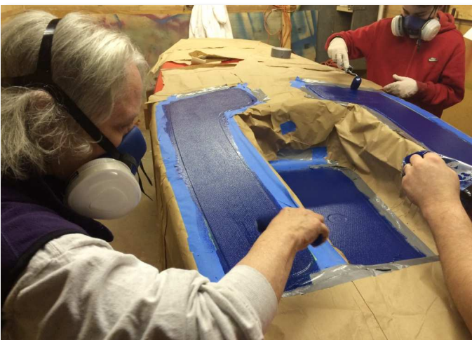
Lynn Anstey (Susquenengo Sqdn.) helps apply non-skid to the deck.
