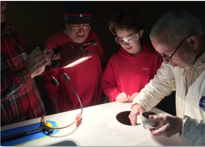
Pat O'Brien, Denis Kingsley, Henry Cabezas and John Read repair a crack in the inner fiberglass skin of the hull.
