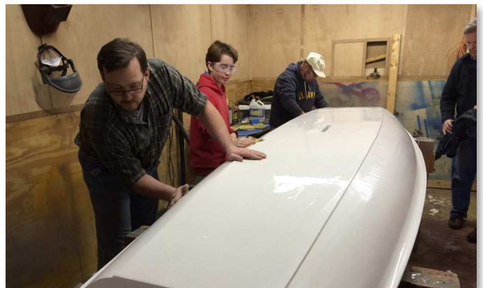
Ben Erway and Henry Cabezas wet sand the bottom following priming and painting.
