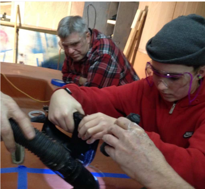
Pat O'Brien looks on as Henry Cabezas cuts a hole in the deck for a new access port.
